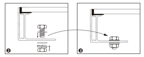
Secure the module in each mounting location with an M8 bolt and a flat washer, spring washer and nut as shown in Figure 1 and tighten to a torque of 16-20 N.m(140-180lbf.in.).
